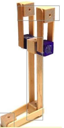
This cube with hole will attach to the end of the piston which actuates the pivot
